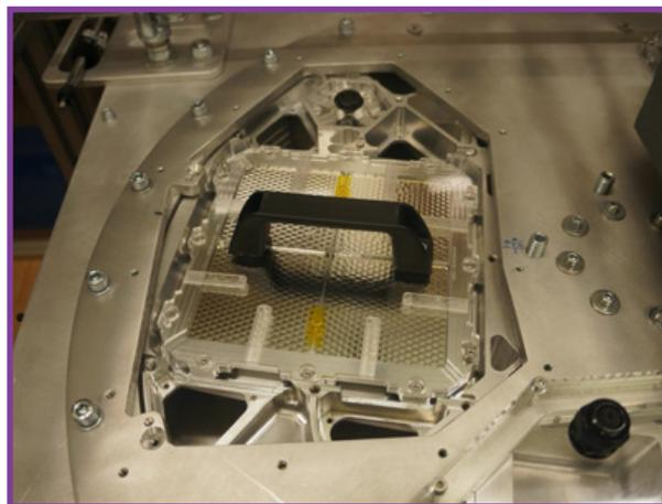
The WFI Thin Filter Assembly (TFA) integrated with a plexiglass handling tool into the Filter Wheel acoustic demonstrator model during the preparation of the acoustic tests at AGH University of Science and Technology in Kraków. Credit: M. Barbera, WFI Consortium.
