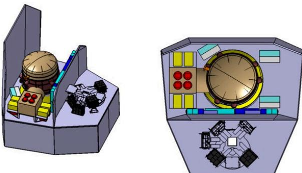
The X-IFU and WFI layouts on the *Athena* Science Instrument Module. The X-IFU design as of December 2019 includes one mini-cryostat accommodating the four Pulse Tube coolers. This is an adaptation of the design presented at the Instrument Preliminary Requirement Review design to specifically reduce perturbations induced by micro-vibrations. This design is still being iterated and likely subject to further modifications. Reference: CNES team (December 2019). Credits: X-IFU Consortium. ©DB/X-IFU.
