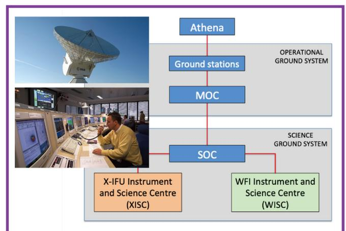
Schematic of the *Athena* Ground Segment (Credit: M. Watson & N. Webb). Top photo: ESA Cebreros antenna (Credit: ESA). Bottom photo: *XMM-Newton* Science Operation Centre (SOC) located at the European Space Astronomy Centre (ESAC) (Credit: ESA).
