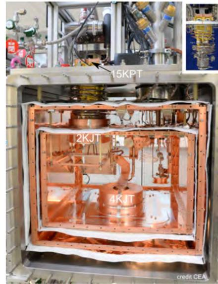
The assembly of the 4K, 2K JAXA Joule-Thomson coolers and the ALAT 15 K Pulse Tube in a laboratory cryostat at CEA-SBT (Grenoble). Courtesy of Thomas Prouvé (CEA/SBT). Credit: CEA/JAXA.
