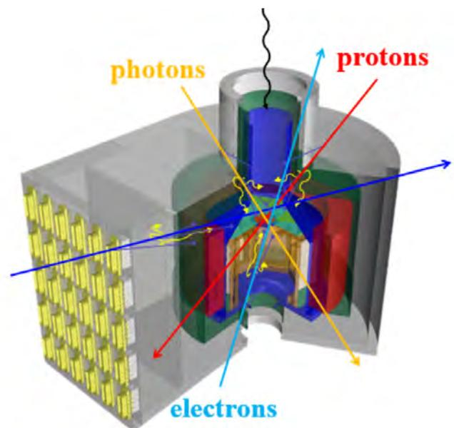
Particle background in a detector. The source photons focused by the optics hit the detector, as the particles (primaries and secondaries) produced by the interaction of the CGR with the satellite. The picture shows the X-IFU FPA (Credit: SRON), but processes are the same for the WFI.
