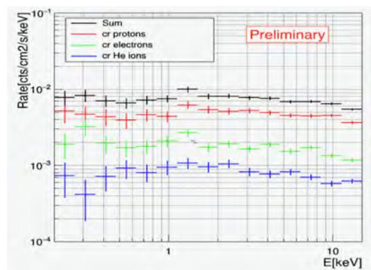
Preliminary spectra of the background in the Athena Instruments. Left - X-IFU background for different configurations of the FPA. Right - WFI background showing contributions from different particle populations (plot courtesy of A. von Kienlin and the WFI team). Optimizations are ongoing for both instruments.
