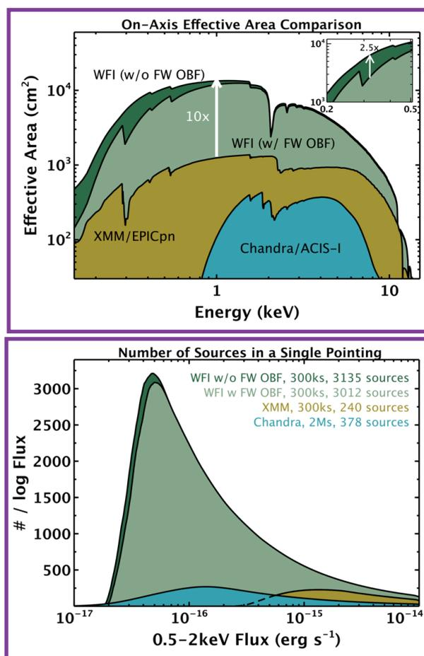
WFI Figures of Merit showing the difference between observations with and without the optical/UV light-blocking filter in the Filter Wheel and in comparison to XMM-Newton and Chandra. Top: Effective Area as function of Energy. The improvement at soft X-ray energies is emphasized in the inset. Bottom: Number of sources detected in a single pointing as function of flux.
