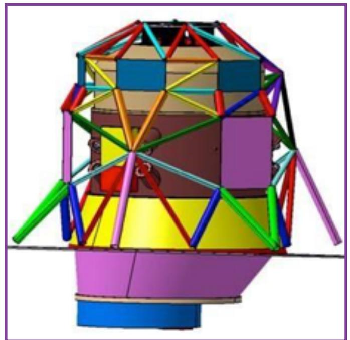
One of the options under study of the new truss structure of the X-IFU Dewar. Courtesy of the CNES project team.
