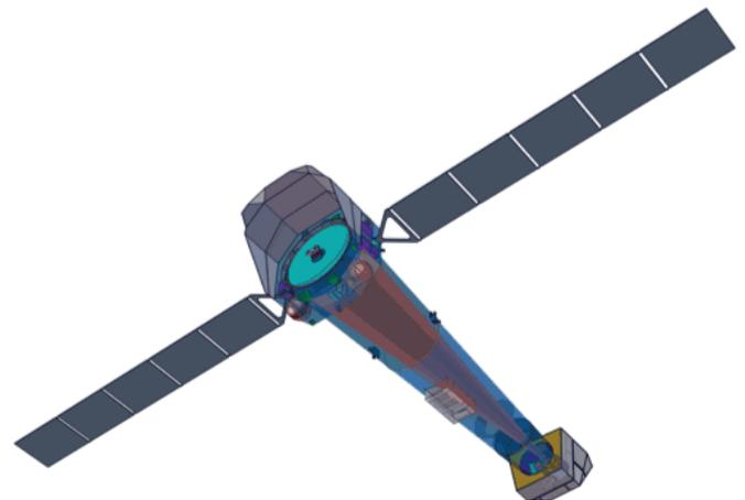
A conceptual design for the Athena spacecraft derived from the ESA CDF study, designed to be accommodated in an Ariane 5 launcher. The Moveable Mirror Array (MMA) is located at the top with the focal plane instruments to the bottom, surrounded by radiators to maintain appropriate thermal control. A fixed optical bench provides the 12m focal length. The spacecraft design has been examined in more detail by the industrial consortia performing the ESA Phase A studies.
