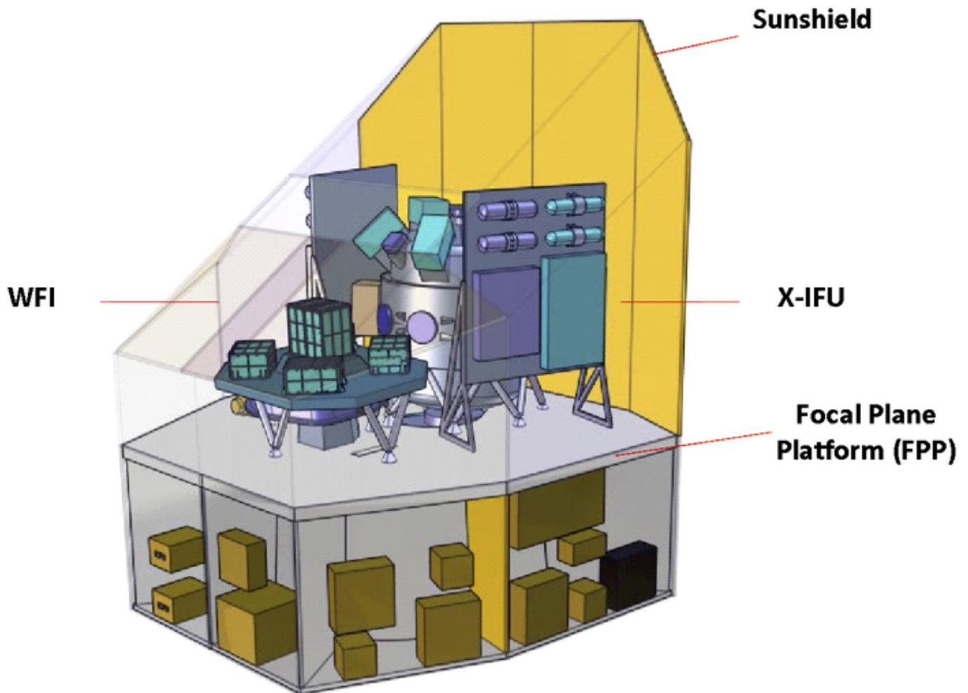
Figure 1: Conceptual design of the Athena Science Instrument Module (SIM), generated from the ESA Concurrent Design Facility (CDF) study undertaken in October/November.
