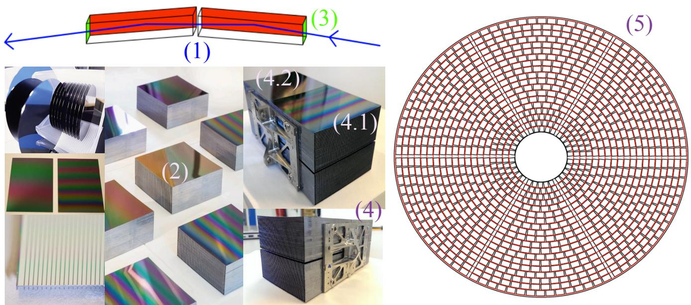
Figure 3: Left: the production of a Mirror Module: ribbed wafers are stacked in an SPO module and 4 are combined in two pairs to form a Mirror Module. Right: front view of the Mirror Assembly Module showing the > 1000 MM required to reach the 2m<sup>2</sup> effective area at 1 keV.
