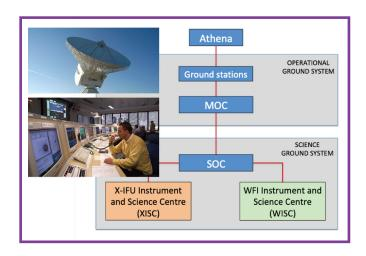
Schematic of the *Athena* Ground Segment (Credit: M. Watson & N. Webb). Top photo: ESA Cebreros antenna (Credit: ESA). Bottom photo: XMM-Newton Science Operation Centre (SOC) located at the European Space Astronomy Centre (ESAC) (Credit: ESA).
