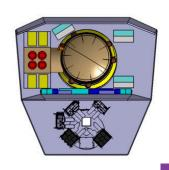
The X-IFU and WFI layouts on the *Athena* Science Instrument Module. The X-IFU design as of December 2019 includes one mini-cryostat accommodating the four Pulse Tube coolers. This is an adaptation of the design presented at the Instrument Preliminary Requirement Review design to specifically reduce perturbations induced by micro-vibrations. This design is still being iterated and likely subject to further modifications. Reference: CNES team (December 2019). Credits: X-IFU Consortium. ©DB/X-IFU.
