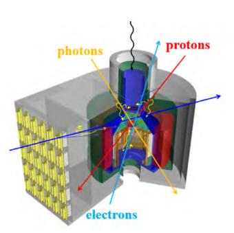
Particle background in a detector. The source photons focused by the optics hit the detector, as the particles (primaries and secondaries) produced by the interaction of the CGR with the satellite. The picture shows the X-IFU FPA (Credit: SRON), but processes are the same for the WFI.
