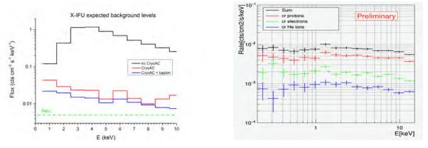
Preliminary spectra of the background in the Athena Instruments. Left - X-IFU background for different configurations of the FPA. Right - WFI background showing contributions from different particle populations (plot courtesy of A. von Kienlin and the WFI team). Optimizations are ongoing for both instruments.
