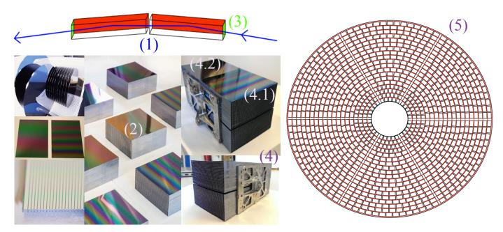
Figure 3: Left: the production of a Mirror Module: ribbed wafers are stacked in an SPO module and 4 are combined in two pairs to form a Mirror Module. Right: front view of the Mirror Assembly Module showing the > 1000 MM required to reach the  $2m^2$  effective area at 1 keV.
