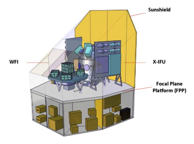
Figure 1: Conceptual design of the Athena Science Instrument Module (SIM), generated from the ESA Concurrent Design Facility (CDF) study undertaken in October/November.
